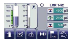
Main screen with intermittent blowdown
